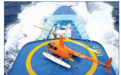
R44 Clipper I shown shipboard with optional rotor blade supports and frame tie-down lugs.
